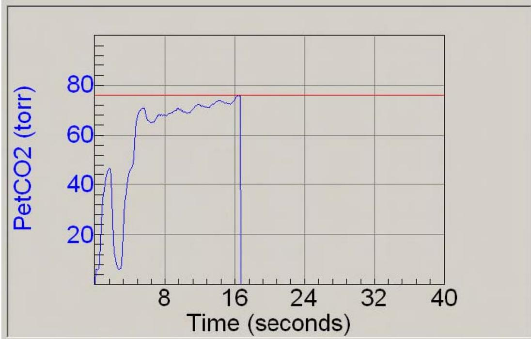
**CO<sub>2</sub> concentration does not equilibrate and continues to rise. CO<sub>2</sub> concentration in the bag is too low and needs to be increased on the next measurement.**
