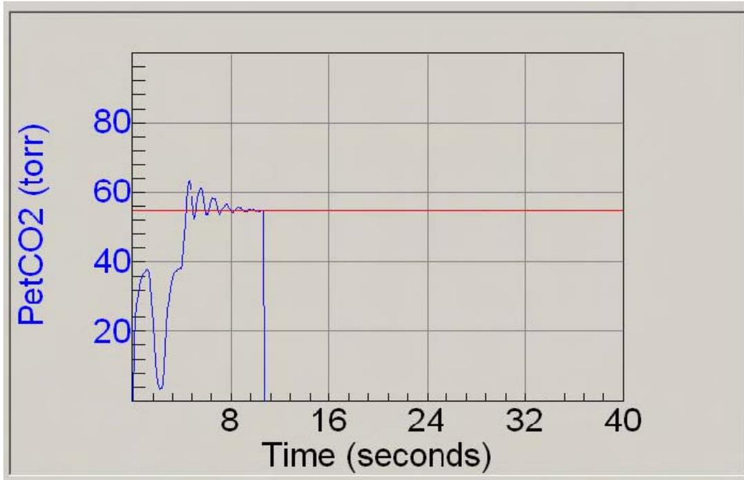
**Acceptable CO<sub>2</sub> curve showing equilibration at the placement of the blue line**
