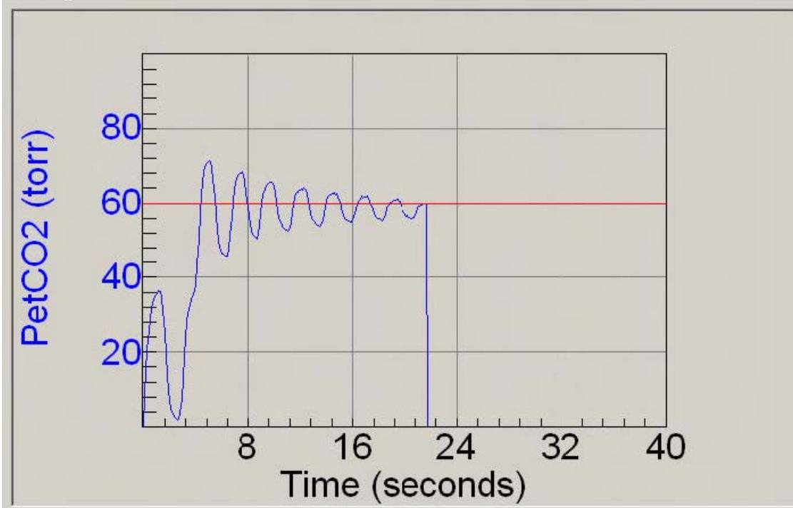
**CO<sub>2</sub> concentration does not equilibrate and continues to oscillate after 10 seconds. CO<sub>2</sub> concentration in the bag is too high and needs to be decreased on the next measurement.**
