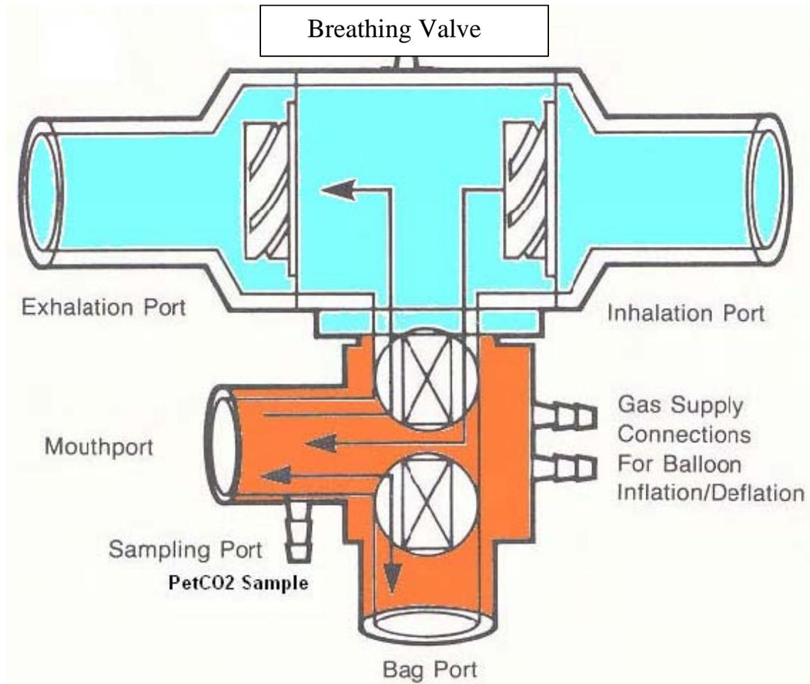
Breathing Valve is shown in blue. Cardiac output valve is shown in orange.
