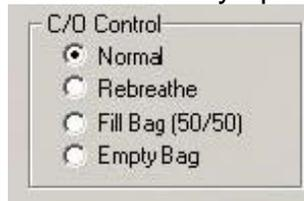
When “Normal” is selected, the lower balloon (the balloon nearest the rebreathing bag) inflates and the upper balloon deflates. The lower balloon should be examined to make sure that it remains fully inflated and does not slowly deflate.
